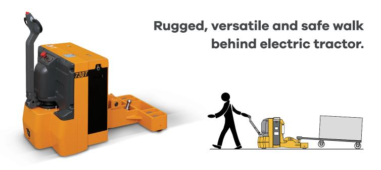
The 730 T are walk behind electric tractors designed as standard for towing trailers of up to 5.0 t and lifting loads of up to 3.0 t. These tractors can be used with different types of trailers. The operator can unlock the hook without releasing the tiller, minimising therefore the handling times.
