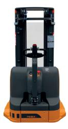
Widened base, ranging from 880 to 1,300 mm and beyond (on request) that can house pallet spars, standard and special containers. Central drive wheel, suitable even for irregular floors
