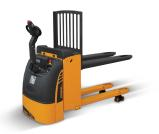
The 316 KN-C and 316 KN-M pallet trucks with mast combine the traditional pallet truck function with the ability to store the load at various height levels. Ideal for safe and comfortable manual load picking and storage in small spaces and on narrow paths, also suitable for overlapped loads.
