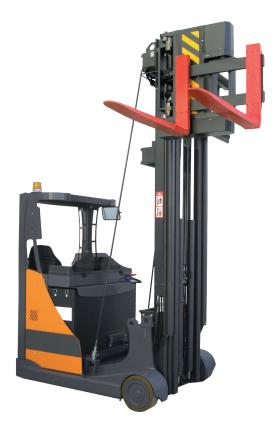
The Neos II TRI ac order picking stacker trucks are designed for transporting and lifting loads in very tight spaces/aisles.
