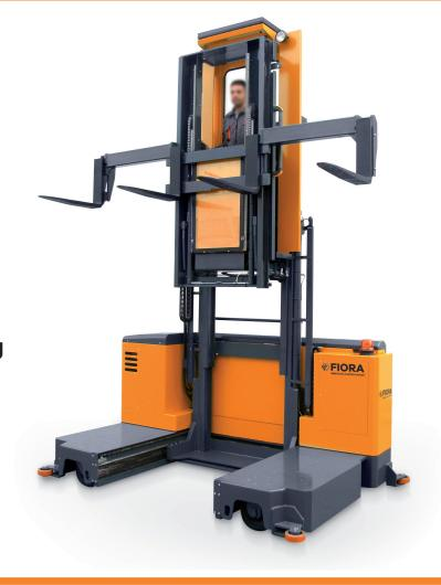
The FIORA I OMG 's order picking side loaders are designed and built for long loads handling. They come with multi-directional drive. Ideal work environments are warehouses aisles and narrow spaces. The philosophy behind our choices is the use of sturdy and cutting-edge materials and components in order to guarantee the safety and reliability of our products even in the most demanding working conditions.
