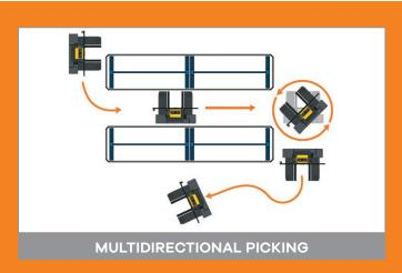
The multi-directional version of the order picking side loader offers the operator the possibility to select the between 6 different driving ways, on both sides. The side loader can steer with the front wheels only or with the rear wheels only, or with all four at the same time. It can also run diagonally and rotate in place, or lock the wheels with the 'in-corridor' guide and improve the working safety of the machine.
