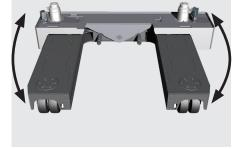
**Polyurethane or cushion rubber wheels**: to work inside warehouses on industrial floors or outside, on paved surfaces. Hydraulic brakes ensure quick response.
