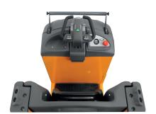
Electronically controlled platform lifting to avoid any jolts. Model 620 PF-S has all the features to ensure highly efficient order picking: fixed platform, load positioned in the vicinity of the operator and a mast with 1000 Kg capacity that can be extended up to a height of 1200 mm.
