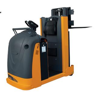
The OMG 620 PF-S ac horizontal order pickers with fixed platform, mast and Fem forks are designed to facilitate first and second level orders picking, representing the ideal combination between productivity and technical performance.
