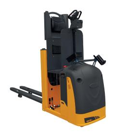
The buttons for slow forward/reverse, backing (optional), are located on both sides of the backrest and are useful for carrying out horizontal movements without climbing back inside the machine.
